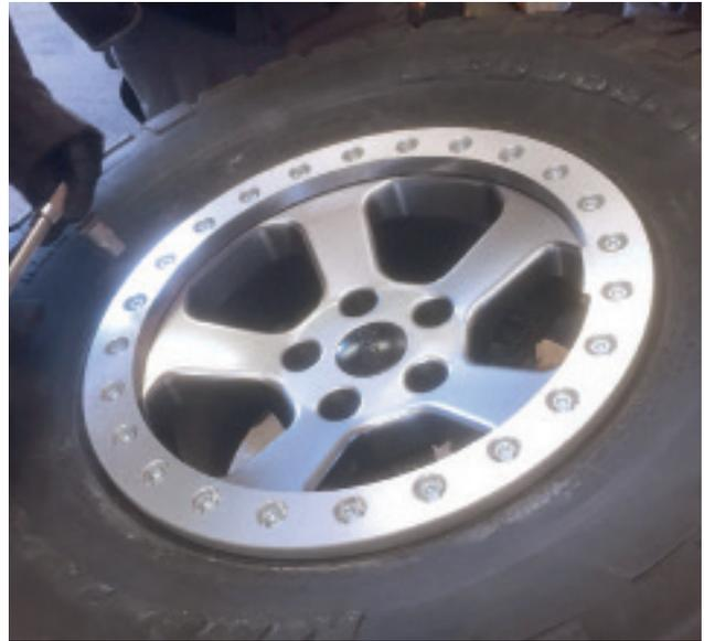
14. This should result in the ring sitting flush on the wheel, or with a small, even gap between the ring and the wheel.
